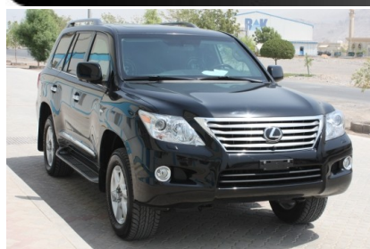
2008 B6 Lexus LX570 (with upgraded blast protection)
